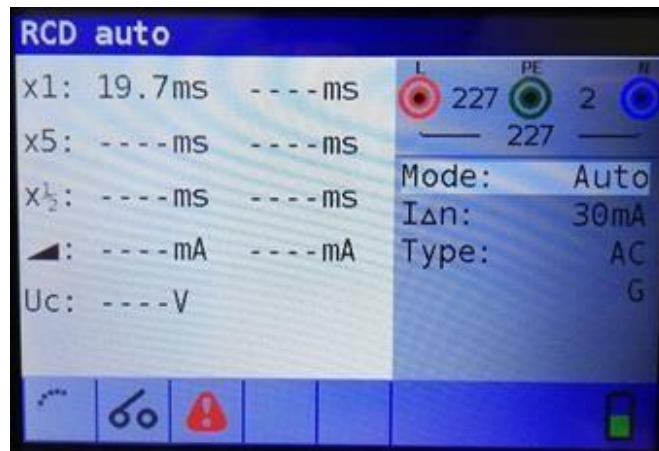
Figure 5-20: Step 1 RCD autotest results
