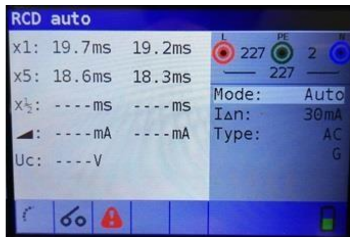
Figure 5-23: Step 4 RCD autotest results
