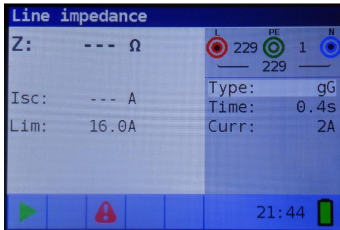
Figure 5-35: Line impedance measurement menu
