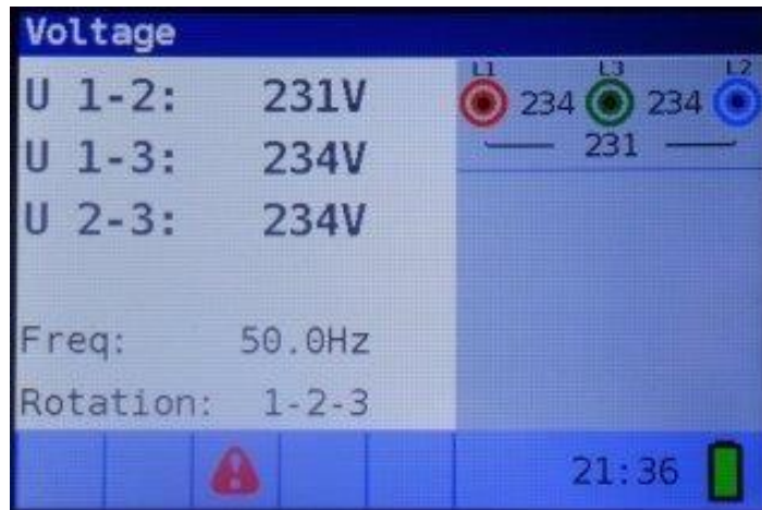
Figure 5-42: Example of phase sequence test result
