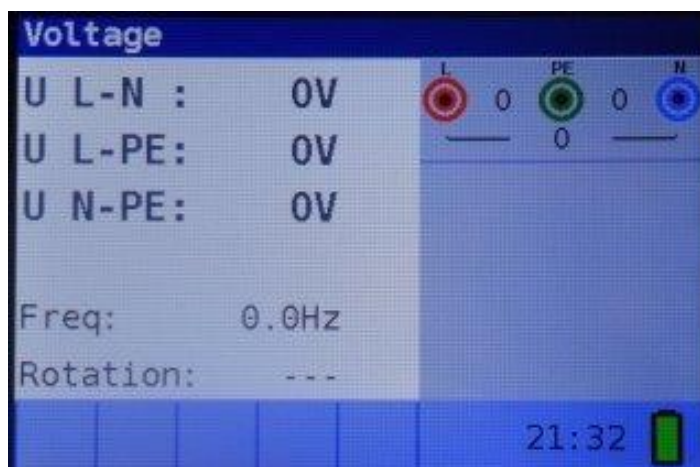
Figure 5-43: Voltage and frequency measurement menu
