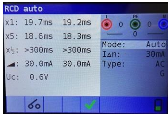
Figure 5-27: Step 8 RCD autotest results
