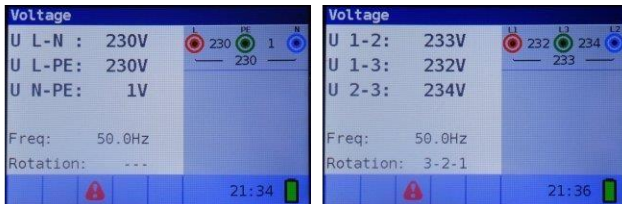
Figure 5-405: Examples of voltage and frequency measurements
